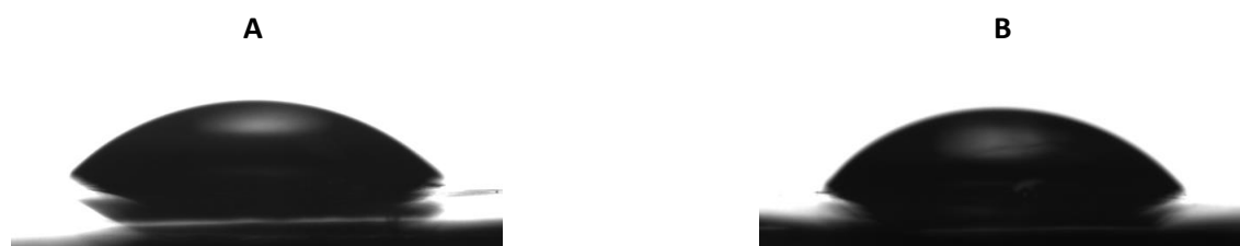
Figure 22 - Contact angle comparison between a fouled membrane ( A ) and a membrane cleaned with an Ultrasil 10 solution ( B ), both from the spiral-wound module.
