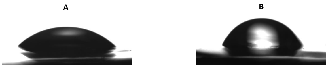
Figure 21 - Contact angle comparison between a fouled membrane ( A ) and a conditioned membrane ( B ), both from the spiral-wound module.
