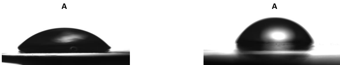
Figure 18 - Contact angle comparison between a fouled membrane (A) and a conditioned membrane (B), both from the flat-sheet batch.
