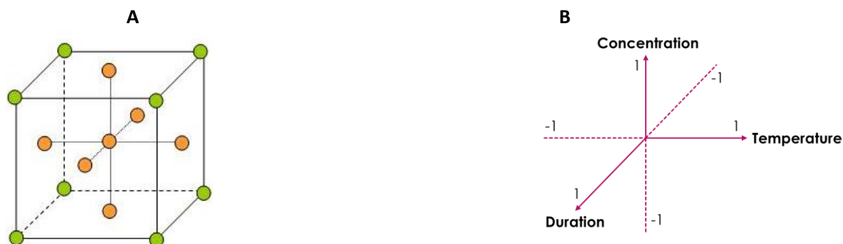
Figure 9 - CCF space design with the data points (A) and the three cleaning factors, represented by three axes (B).
